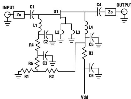
Figure 1. Typical ATF-55143 LNA with Passive Biasing.
