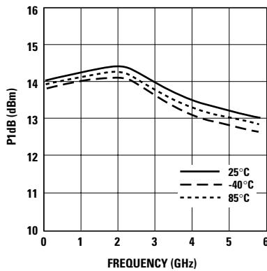
Figure 25. P1dB vs. Temperature and Frequency with bias at 2.7V, 10 mA.<sup>[1,2]</sup>
