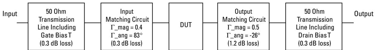
**Figure 5. Block diagram of 2 GHz production test board used for Noise Figure, Associated Gain, P1dB, OIP3, and IIP3 measurements. This circuit represents a trade-off between an optimal noise match, maximum OIP3 match and associated impedance matching circuit losses. Circuit losses have been de-embedded from actual measurements.**
