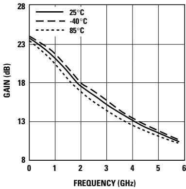
Figure 21. Gain vs. Temperature and Frequency with bias at 2.7V, 10 mA.<sup>[1]</sup>
