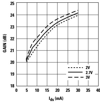
Figure 16. Gain vs.  $I_{ds}$  and  $V_{ds}$  at 900 MHz.<sup>[1]</sup>
