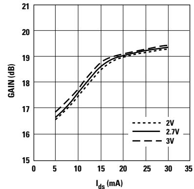
Figure 11. Gain vs.  $I_{ds}$  and  $V_{ds}$  at 2 GHz.<sup>[1,2]</sup>
