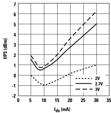
Figure 19. IIP3 vs.  $I_{ds}$  and  $V_{ds}$  at 900 MHz.<sup>[1]</sup>
