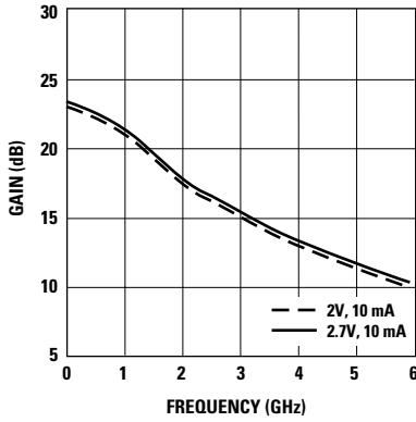
Figure 6. Gain vs. Bias over Frequency.<sup>[1]</sup>
