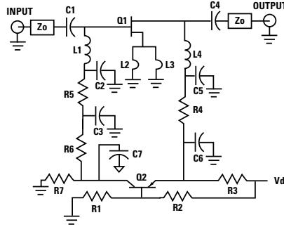
Figure 2. Typical ATF-55143 LNA with Active Biasing.
