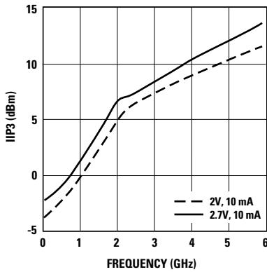
Figure 9. IIP3 vs. Bias over Frequency.<sup>[1]</sup>
