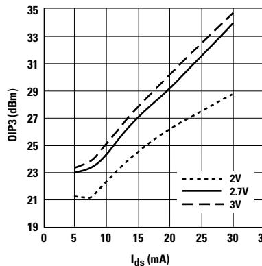
Figure 13. OIP3 vs.  $I_{ds}$  and  $V_{ds}$  at 2 GHz.<sup>[1]</sup>
