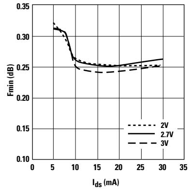
Figure 17.  $F_{min}$  vs.  $I_{ds}$  and  $V_{ds}$  at 900 MHz.
