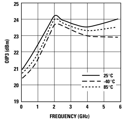
Figure 23. OIP3 vs. Temperature and Frequency with bias at 2.7V, 10 mA.<sup>[1]</sup>
