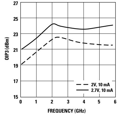
Figure 8. OIP3 vs. Bias over Frequency.<sup>[1]</sup>
