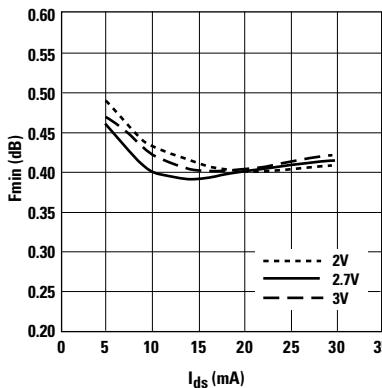
Figure 12. Fmin vs.  $I_{ds}$  and  $V_{ds}$  at 2 GHz.
