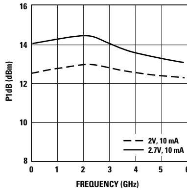
Figure 10. P1dB vs. Bias over Frequency.<sup>[1,2]</sup>
