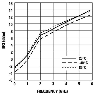
Figure 24. IIP3 vs. Temperature and Frequency with bias at 2.7V, 10 mA.<sup>[1]</sup>
