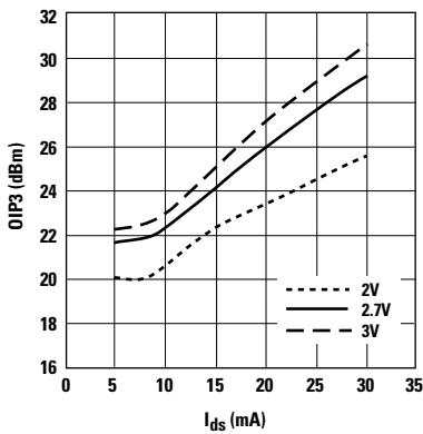
Figure 18. OIP3 vs.  $I_{ds}$  and  $V_{ds}$  at 900 MHz.<sup>[1]</sup>
