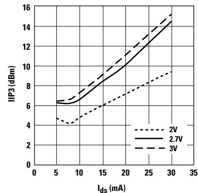
Figure 14. IIP3 vs.  $I_{ds}$  and  $V_{ds}$  at 2 GHz.<sup>[1]</sup>
