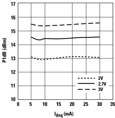
Figure 15. P1dB vs.  $I_{dsq}$  and  $V_{ds}$  at 2 GHz.<sup>[1,2]</sup>
