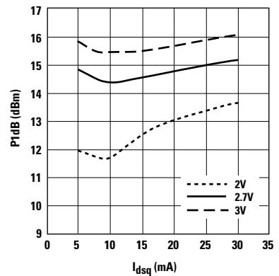
Figure 20. P1dB vs.  $I_{dsq}$  and  $V_{ds}$  at 900 MHz.<sup>[1,2]</sup>
