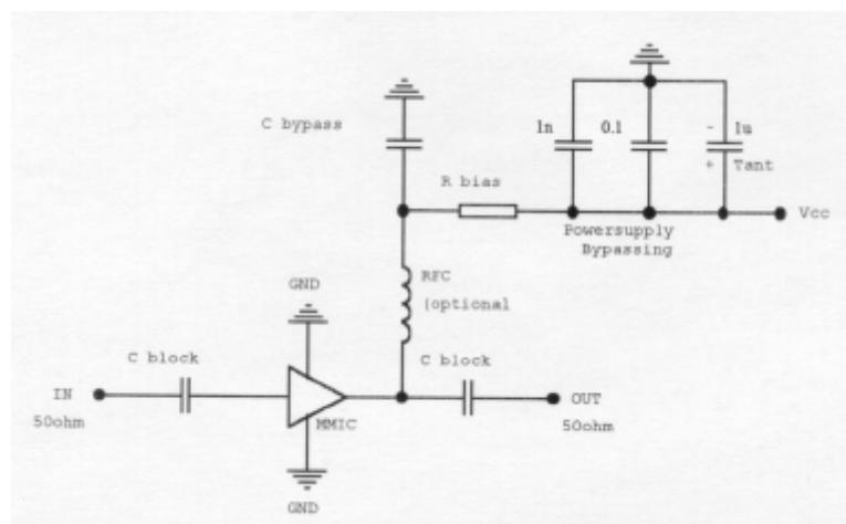
$$R_{\text{bias}} = \frac{V_{\text{cc}} - V_d}{I_{\text{bias}}}$$
